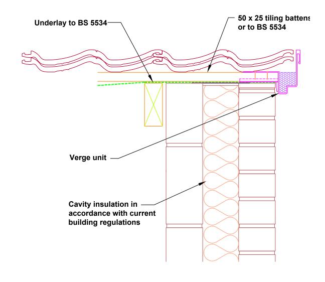
Note: When using a vapour permeable (LR) underlay, Forticrete in line with BS5250 recommend that the batten cavity is ventilated from eave to ridge
